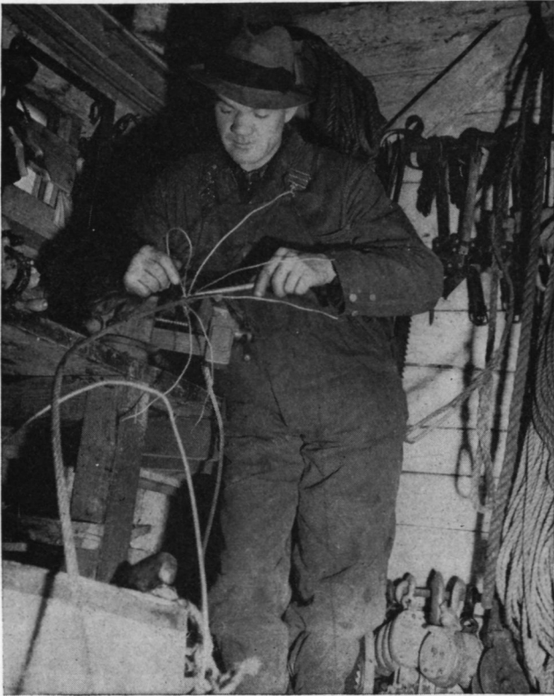
FIG. 3.107. Inside a rigger's hut during a steel-rope splicing operation. Notice typical rigging equipment in background.
